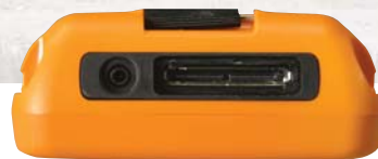
Multi-Interface and Power/Charge connectors mounted in a shock absorbing, rubber retainer
