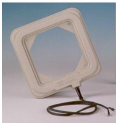
At the start of the line, BSC affixes an RFID tag to the seatback and "registers" it with a tag reader. Next, the airbag serial number is scanned, and the seatback assembly is then matched with a seat bottom to form a single production unit. At each stage in the assembly process, an antenna reads the RFID tag to identify the seat being built. Lot numbers and safety-related data, including quality checks and torque readings, are recorded.
